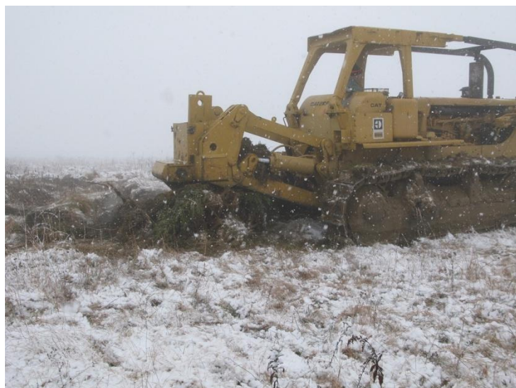
Figure 2: Dozer "deep ripping" at Barton Bench to prepare ground for planting red spruce.
